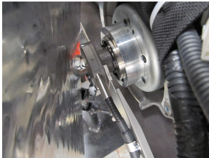
Figure 4.6: Crank angle encoder attached to the magneto
